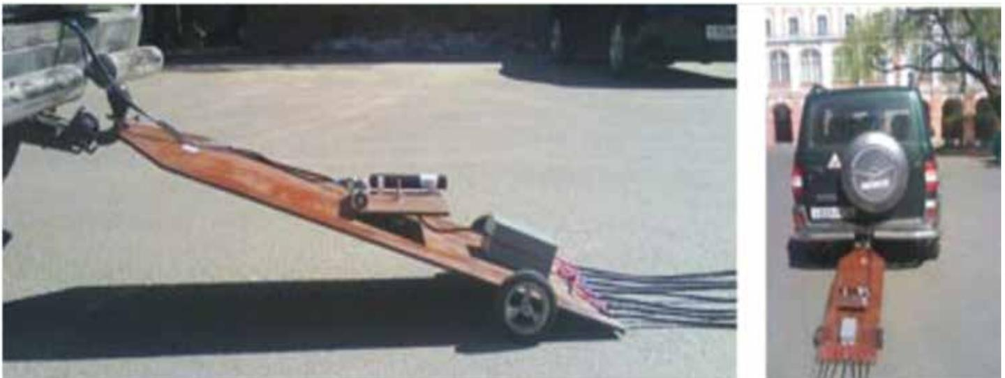
**Figure 12.** Measuring block formed by two horizontal magnetic antennae, electric signal preamplifier and electric antenna (Simakov et al., 2010).
