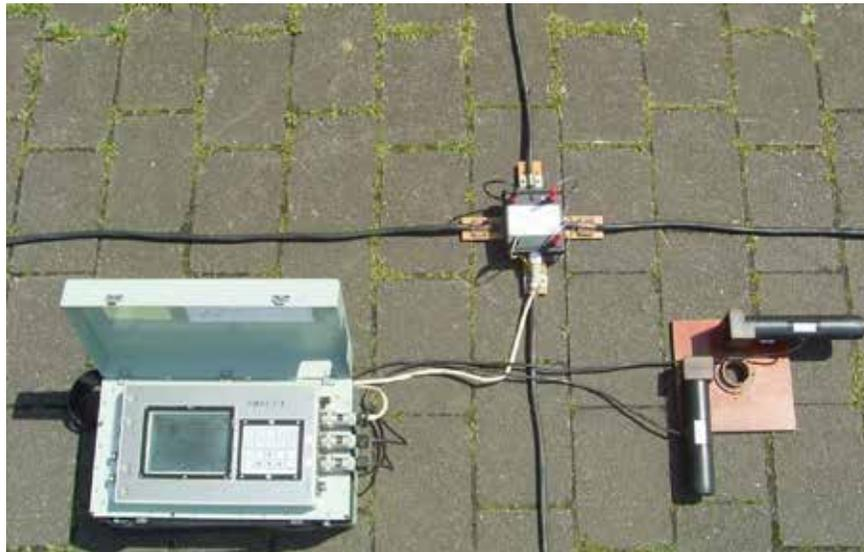
**Figure 6.** The new digital RMT-F1 system (Tezkan, 2009).
